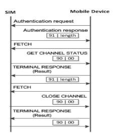
Fig. 3. SIM-ME interactions to drop the established connection
